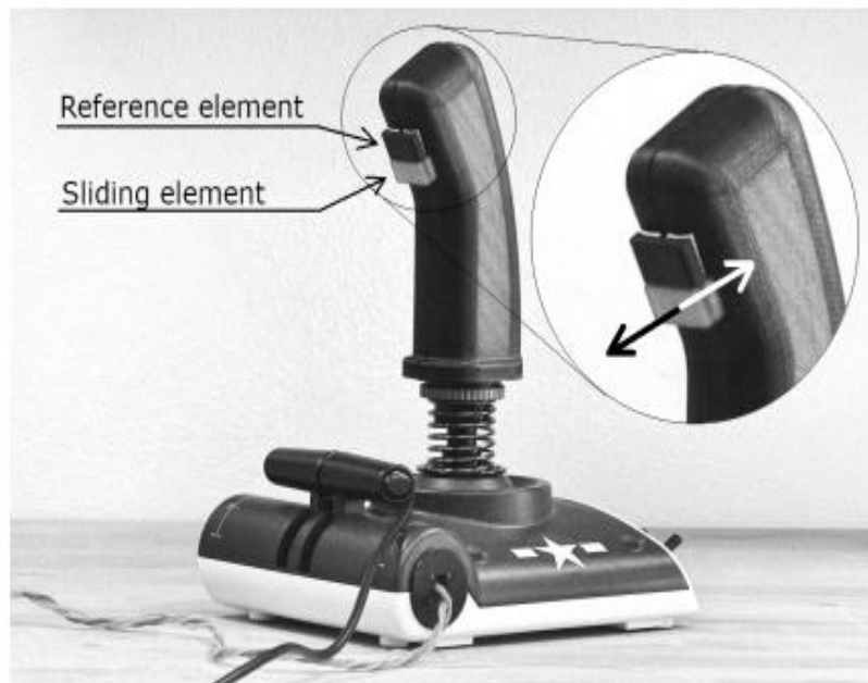
Fig. 1 Joystick with tactile guidance device attached [2]
