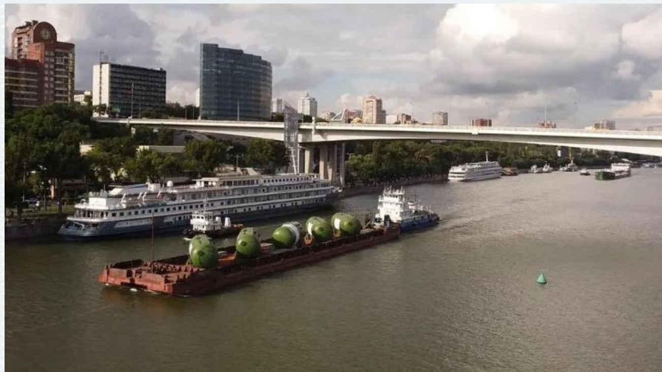
"Atommash transportation of steam generator for Bangladesh" by YuliaTikhonova is licensed under CC BY-SA 4.0 .
