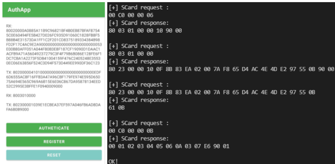
Figure 2: Smart phone application screen (left side) and log of successful authentication (right side).
