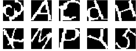
Fig. 5: Sample output from segmentation stage (characters a, A, C, d, H, k, M, P, Y and 5)
